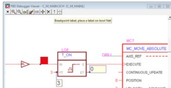
Graphical debugging with breakpoints, live labels and highlighting active Nets and Function Blocks
